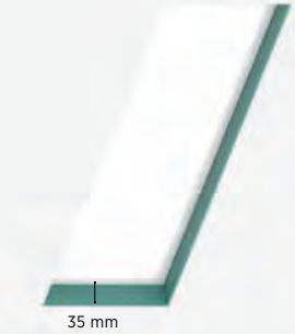
WHITELINE + KORONA EFFECT: with coloured recessing frame; 35 mm back shifted into the ceiling (colour No. 20 - „Poseidon's Paradise“)
